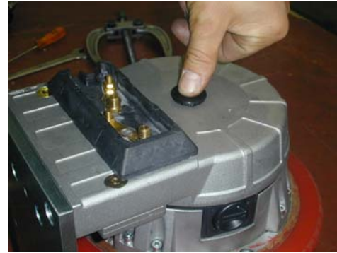
15. Insert sealing plug into borehole
