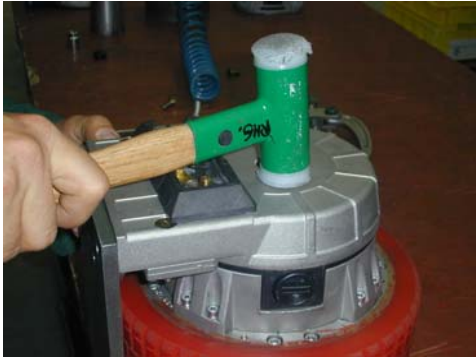
13. Place brush flange and drive in straight onto the engine shaft
