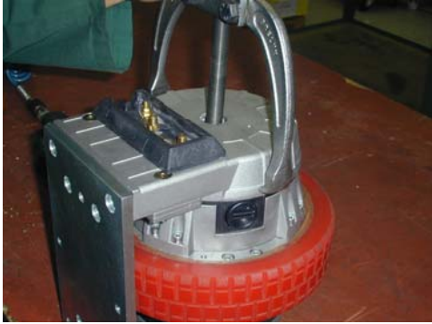
5. Pull brush flange off the engine axle
